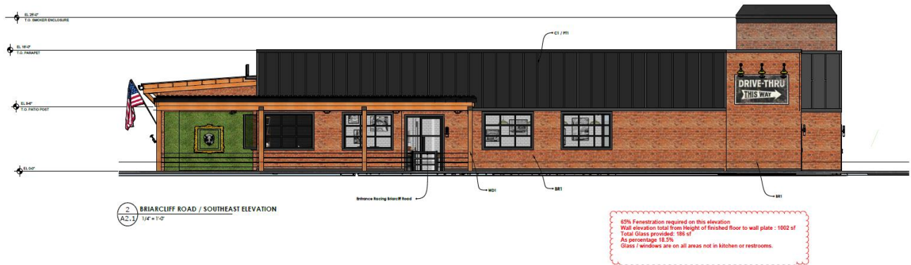
Figure 6. Proposed southern building façade fronting Briarcliff Road. Note on the plan indicates 18.5 percent fenestration along this façade, and “glass/windows are on all areas not in kitchen or restrooms.”
