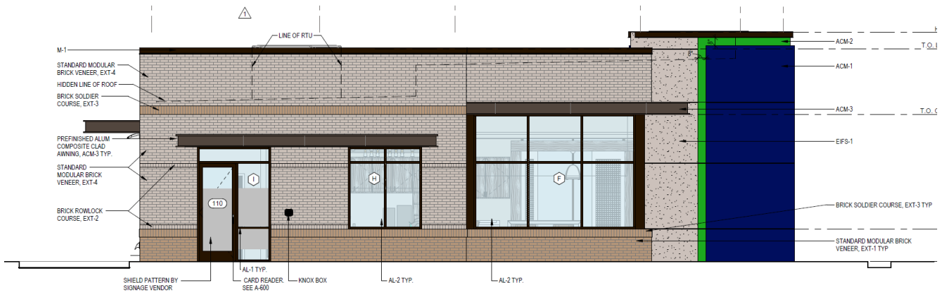
Figure 6. Montreal Road Elevation with 32.7% Fenestration.
